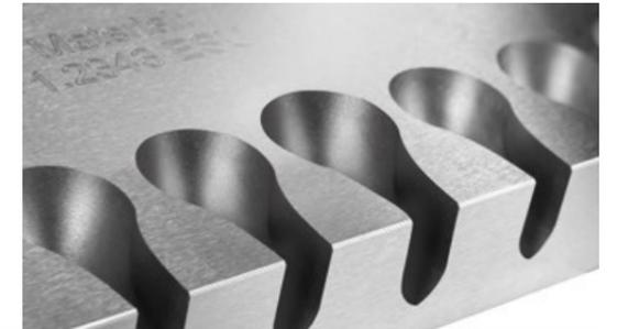
Precision and cost-effectiveness are especially important in multi-cavity machining. The new *EAGLE* PowerSPARK Generator reduces wear by up to 50%, due to the unique adaptive pulse form, now also in finishing.
